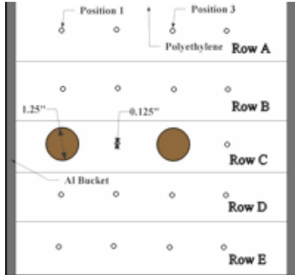
FIGURE 2: Polyethylene configuration for SER irradiations in the RSEC FNI
